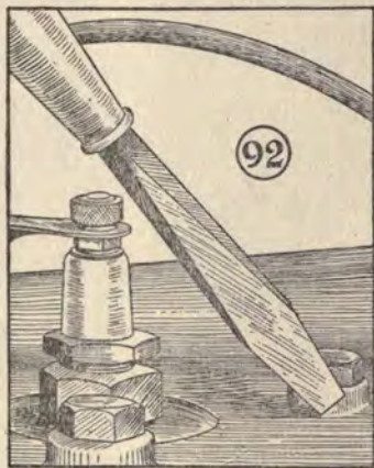
Fig. 92—Spark plugs are tested with a screwdriver by shorting them to the cylinder block
