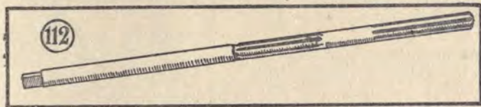
Fig. 112—Spindle bushing reamer which reams the two bushings so that they are in perfect alignment
