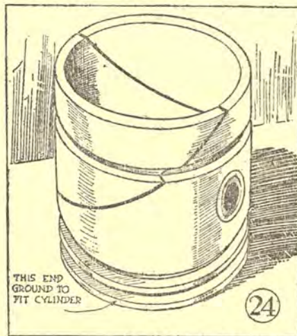
Fig. 24—An old piston slit to make a cylinder lap
