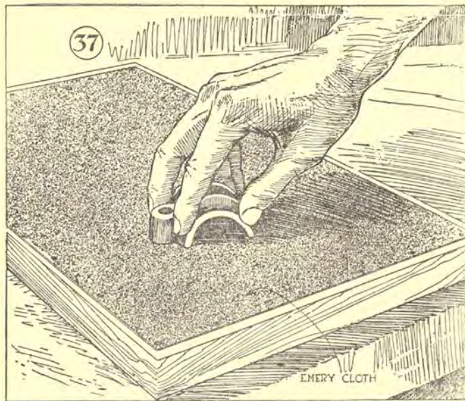
Fig. 37—Both the main bearing and connecting-rod caps are taken down on emery cloth
