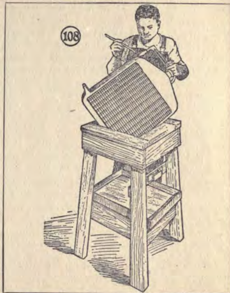
Fig. 108—This is a handy stand for soldering and working on a radiator
