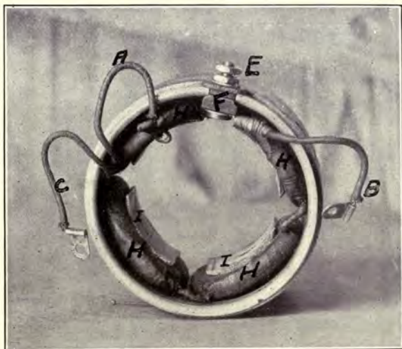
FIGURE 3. LOOKING AT GENERATOR FRAME WITH END HOUSING REMOVED.
